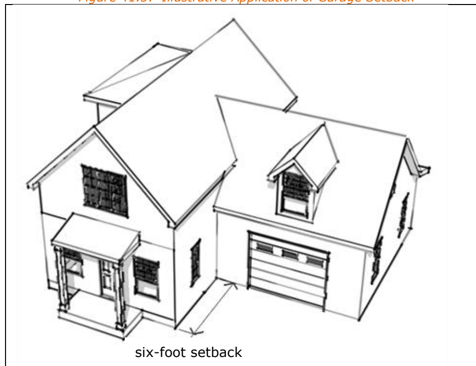
Figure 41.3: Illustrative Application of Garage Setback
